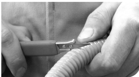
Step 1: Cut through the plastic mantle, if present.
