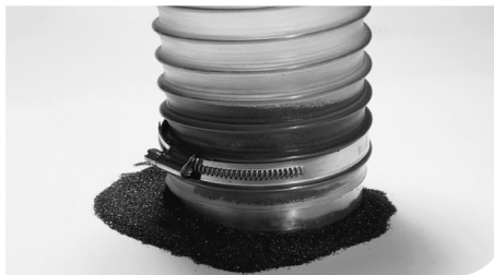
Significant leakage when using conventional hose clamps.
