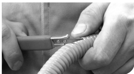
Step 1: Cut through the plastic mantle, if existing.
